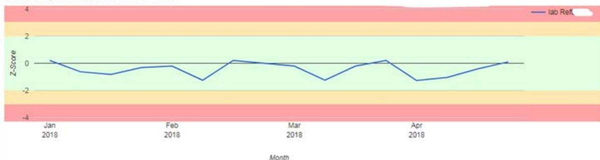
Reference labs can also produce these reports. Here the reference result for Dumas N is slightly low over time vs the assigned value.
