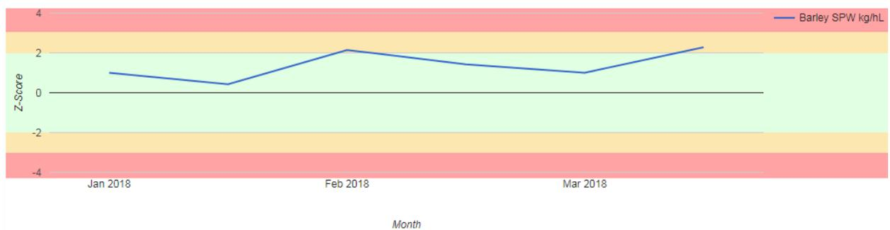
Here is an example of a report generated by selecting a specific test on a specific subscription. We can see that the instrument is showing signs of positive bias. There are few z score failures but all the results are positive.
