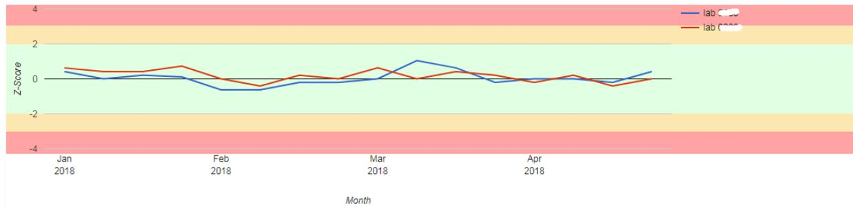
Here we have an example generated by selecting a lab with two subscriptions, both submitting data for Barley Nitrogen. Both instruments are showing excellent performance with the lines close to and centred around zero.
